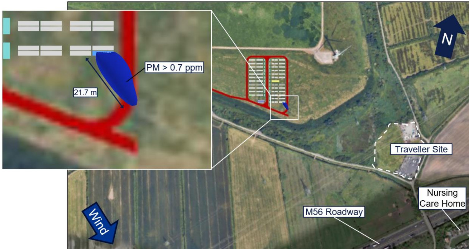
Figure A 9: Case 101 – Particulate Matter Plot with Wind from NW at 5 m/s
