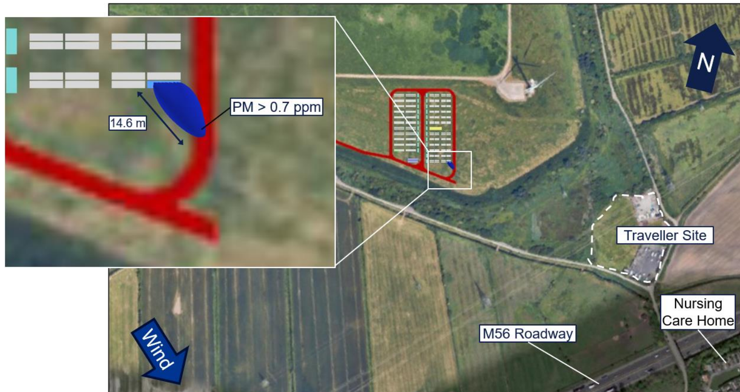
Figure A 10: Case 102 – Particulate Matter Plot with Wind from NW at 10 m/s
