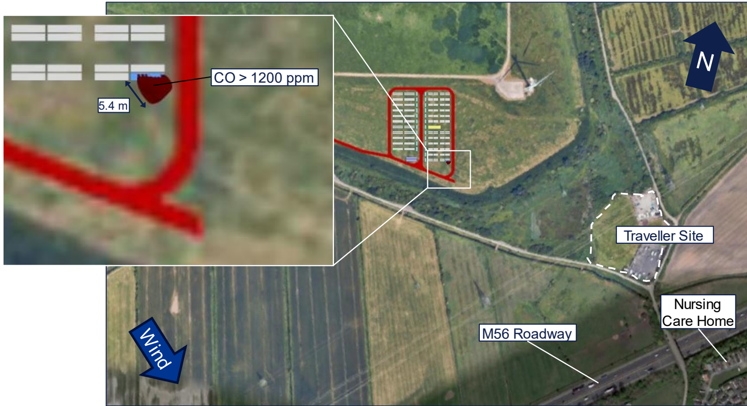
Figure A 5: Case 101 – Carbon Monoxide Plot with Wind from NW at 5 m/s
